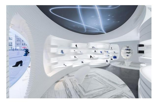
The sinuous walls are clad with HI-MACS® acrylic stone in the Alpine White shade. Continuing the play of lines in the walls, the displays are fashioned from thinner layers of translucent HI-MACS® Opal, backlit with LEDs.
